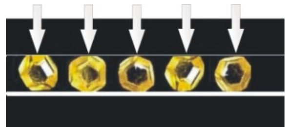
Fig. 2: Illustrating Multiple Points of Contact using Graded Diamond Powder Resulting in Improved Surface Finish.
