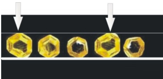
Fig. 1: Illustrating Limited Points of Contact Ungraded Diamond Powder Resulting in Scratch Formation
